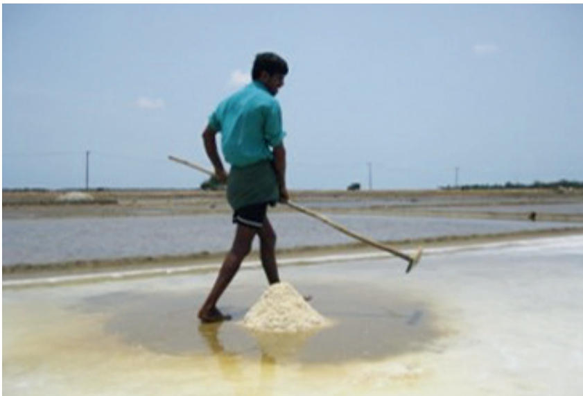
Solar salt crystallizes in a pond, and once it reaches appropriate density, it can be harvested and washed in brine to remove impurities.
