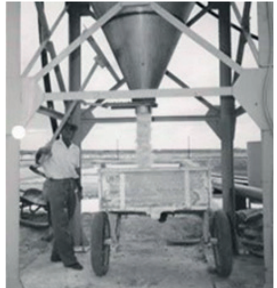
An early salt washing system patented in the U.S. in 1963, here being used in a salt pond in South Africa. The apparatus is mobile thanks to wheels, and the hopper can be moved from pond to pond. Salt is loaded and washed with brine, and it lands on stockpiles to dry.
